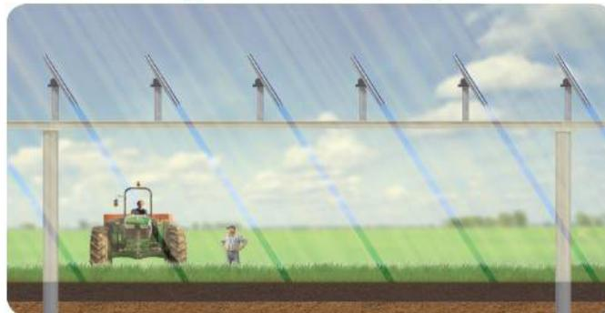
The opposite of Normal Tracking where panels are parallel to the sunlight allowing maximum sunlight on crops
