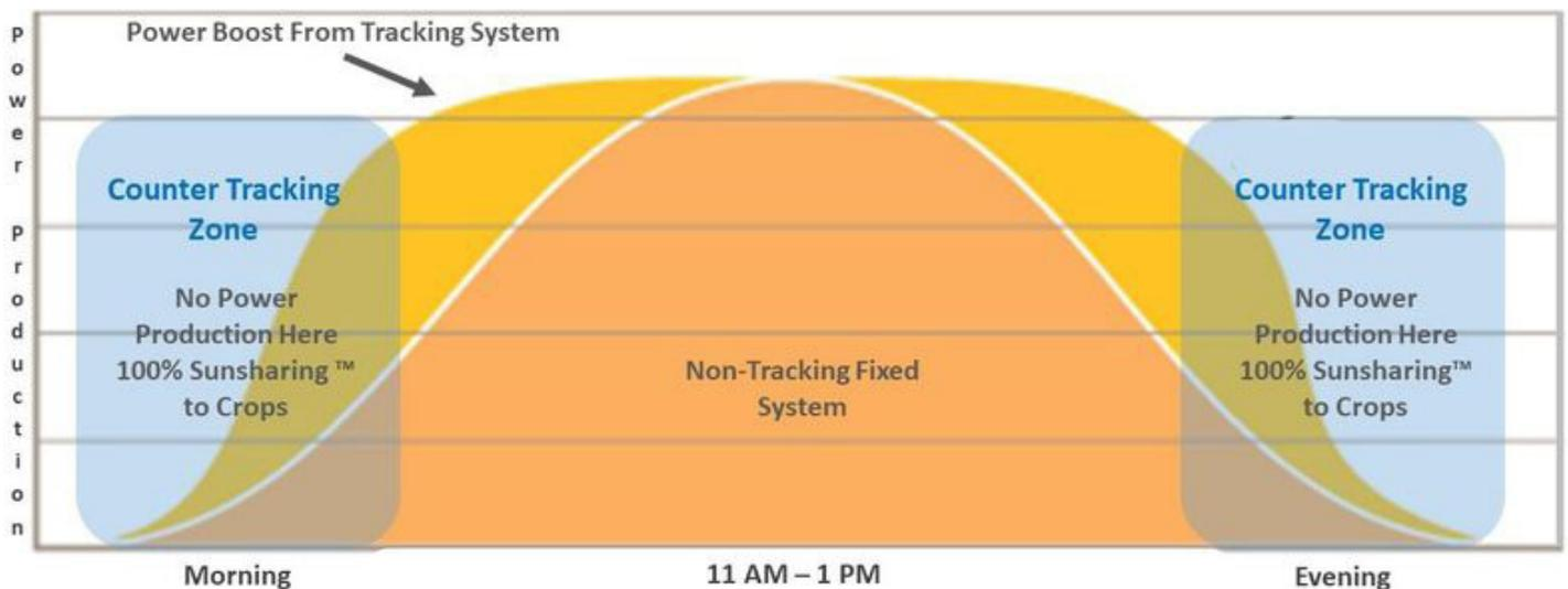
Note 1: The counter tracking zones are not a fixed size, they can be as large or as small as the producer chooses.
