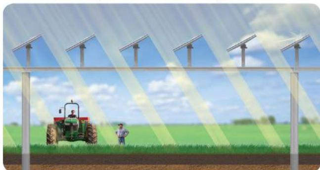
Solar panels are perpendicular to the sunlight and provide partial shading
