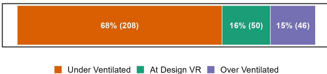
Figure 1.7. Percentage of classrooms at, above and below design ventilation rate as per ASHRAE Standard 62.1.
