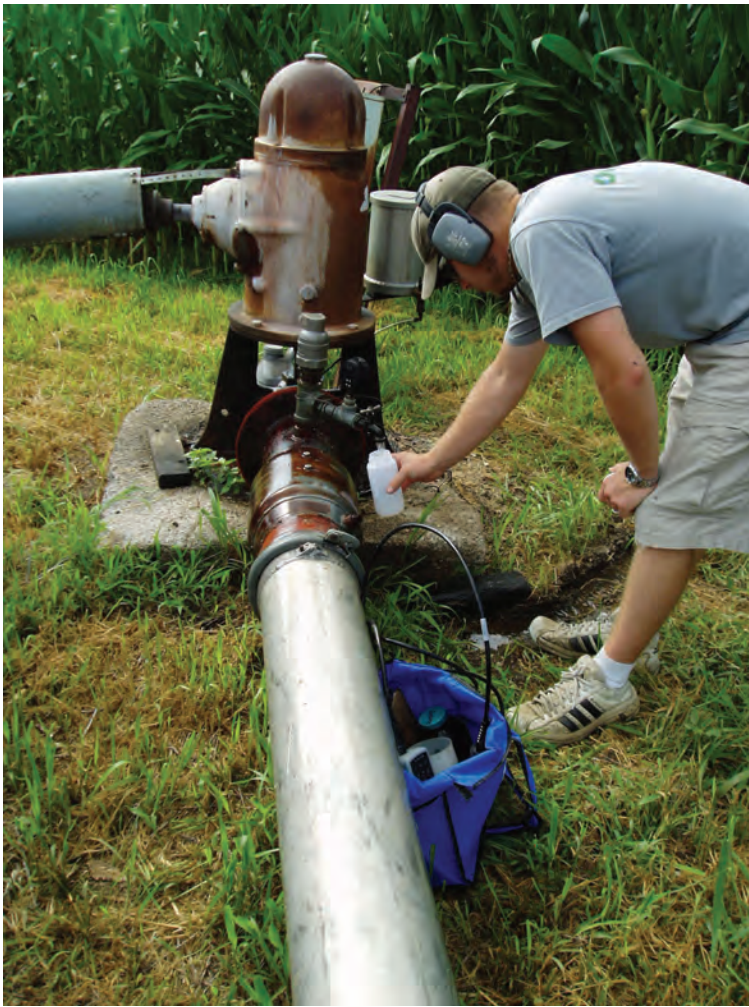
Lower Platte South Natural Resources District staff sampling an irrigation well.
