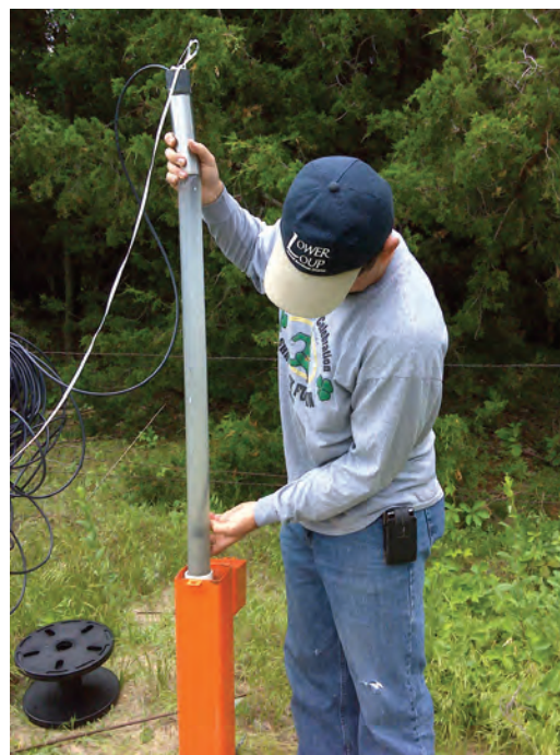
Lower Loup Natural Resources District staff utilizing a passive diffusion sampler to sample a monitoring well near Duncan, NE.
